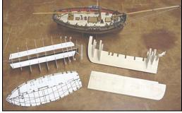
Mitchell stated that one area where his technique caused problems was along the transom. The curve and angle of that surface did not allow the true shape to be projected in any view, and John was required to work at it until he obtained the correct form.
